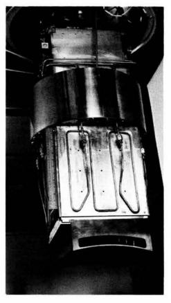
NOW ON SITE at the TEXTOR in West Germany, this Advanced Limiter Test Module may lead to new ways to remove heat and particles from magnetic fusion devices.
